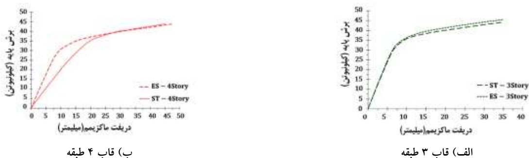
Fig. 8. Base shear diagrams in terms of maximum in-plane relative displacement for partial connections
