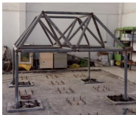
Fig. 2. The double layer Grid made in a Laboratory
