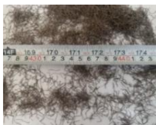
Fig. 1. Micro recycled steel fibers
