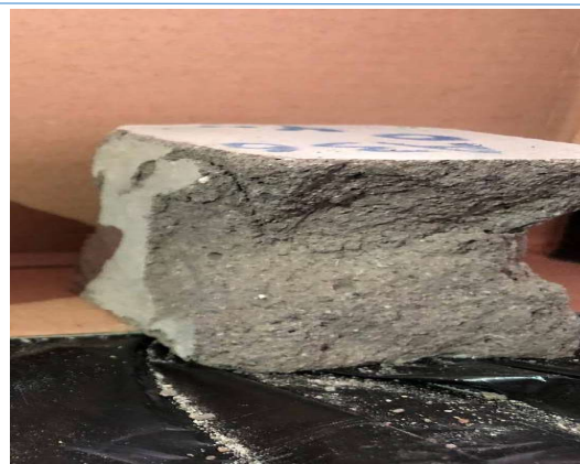
Fig. 10. The appearance of R2F12G0.5 design sample after 600 degree temperature
