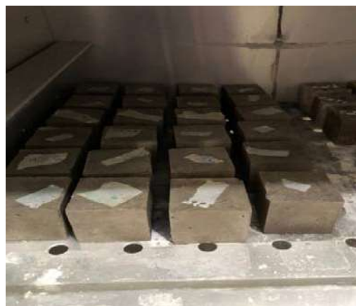
Fig. 1. The arrangement of the samples in the furnace under the heat of 200 degree
