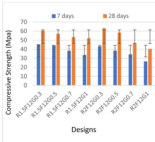
Fig. 3. compressive strength of 7 and 28 days samples
