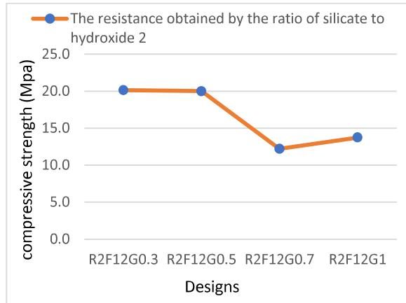
Fig. 5. Gained resistance at ratio 2 between 7 and 28 days
