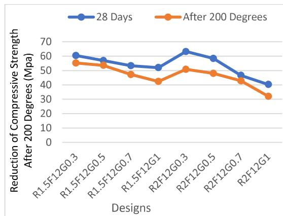
Fig. 7. Reduction of strength after 200 degree heating
