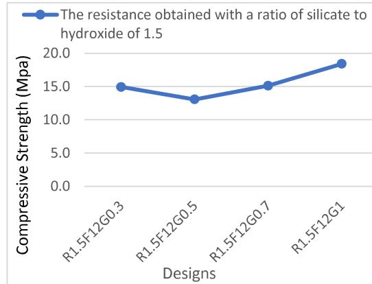
Fig. 4. Gained resistance at ratio 1.5 between 7 and 28days
