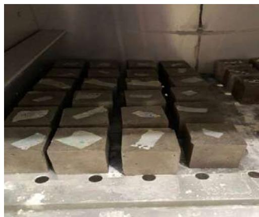
Fig. 1. The arrangement of the samples in the furnace under the heat of 200 degree
