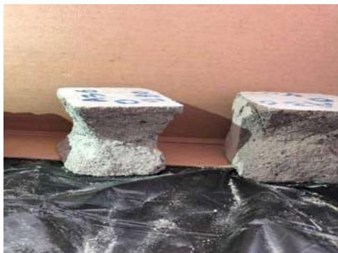
Fig. 9. The appearance of R2F12G0.5 design samples after exposure to high temperature
