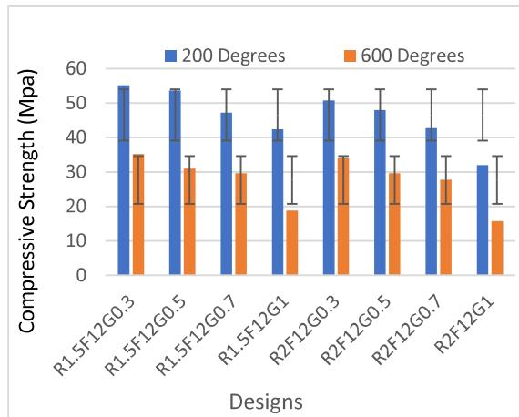
Fig. 6. Compressive strength after 200 and 600 degrees heating
