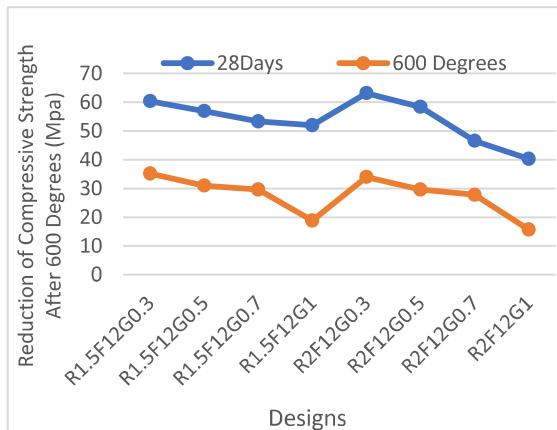
Fig. 8. Reduction of strength after 600 degree heating
