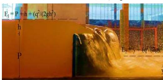
Fig. 1. Parameters affecting energy loss
