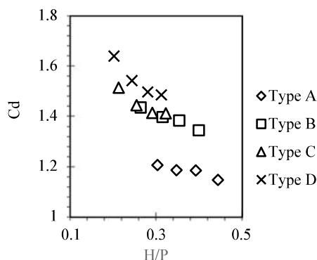
Fig. 7. The water passage coefficient of the sinusoidal labyrinth weir
