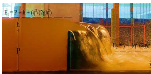
Fig. 1. Parameters affecting energy loss
