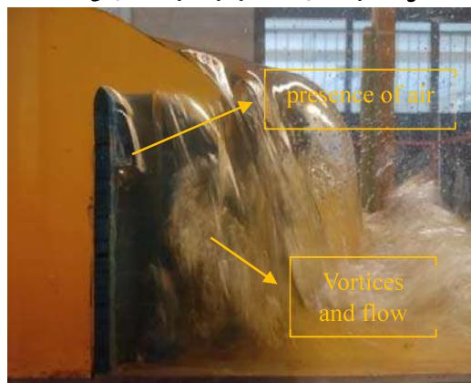
Fig. 4. Flow in the sinusoidal labyrinth weir
