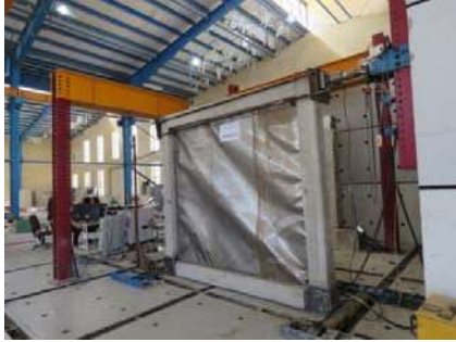
Fig. 10. Sample after loading up to 2.02% displacement
