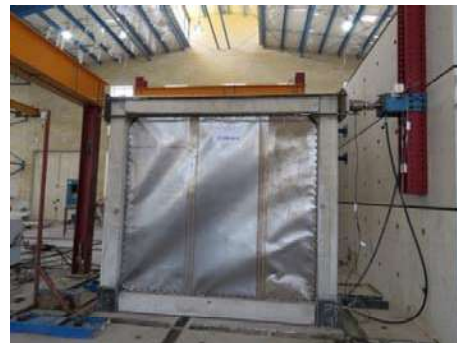
Fig. 8. Occurrence of permanent buckling of web sheet in displacement of 1.5%
