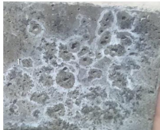
Fig. 3. Sample taken out of sodium sulfate solution
