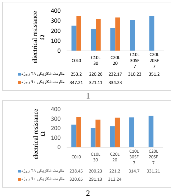
Fig. 6. electrical resistance test for 28 and 90 day samples 1: with a ratio of water to cement materials of 0.35 and 2: with a ratio of water to cement materials of 0.4
