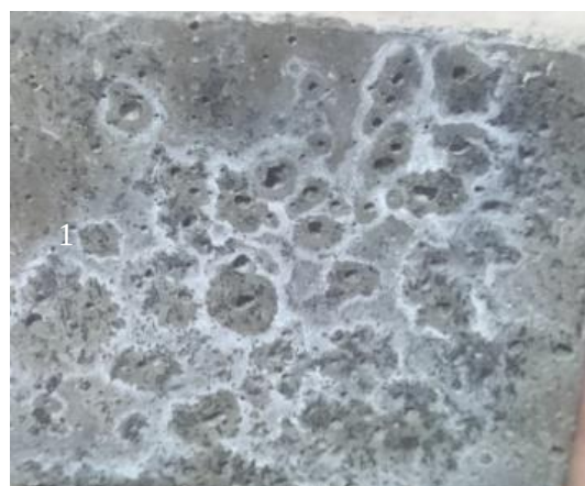
Fig. 3. Sample taken out of sodium sulfate solution
