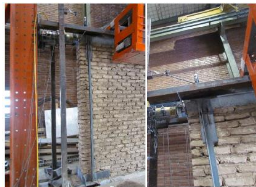
b) Adopted details for controlling the uplift in the wall
