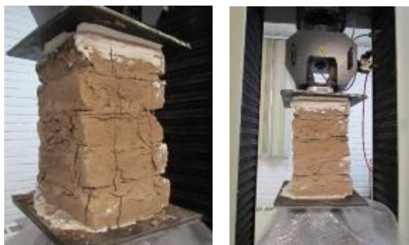
Fig. 6. Compressive strength test on adobe prism
