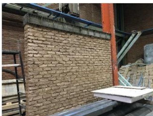
Fig. 5. The wall specimen and the top RC beam
