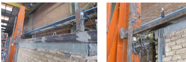
Fig. 10. Adopted instruments for measuring displacement
