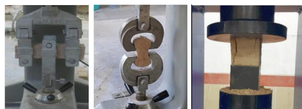
Fig. 4. Set-up for compressive, tensile and flexural strength tests of clay mortar
