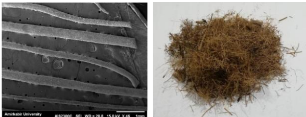
Fig.3. Palm fibers and their microscopic picture [7]
