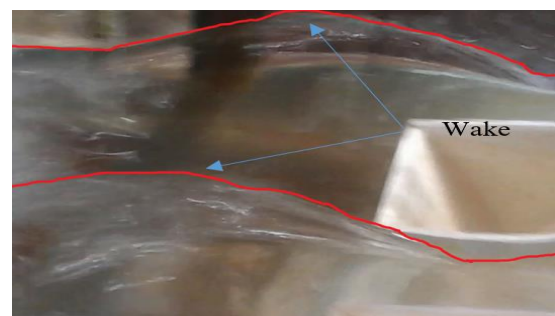
Fig. 4. Flow disturbance on the weir
