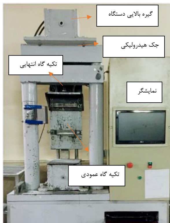
Fig. 3. Single-lap shear test setup
