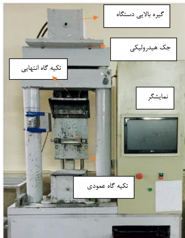
Fig. 3. Single-lap shear test setup
