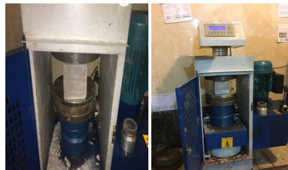
Fig. 3. Compressive strength test on RPC samples
