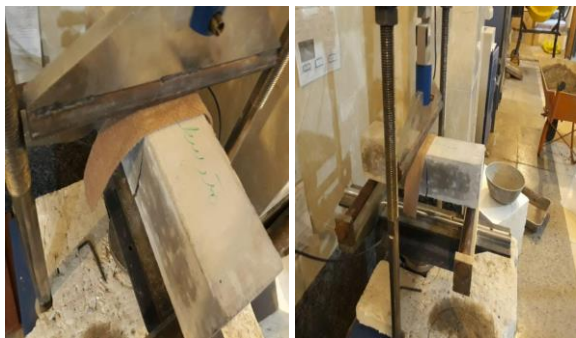
Fig. 4. Bending strength test on RPC concrete beam
