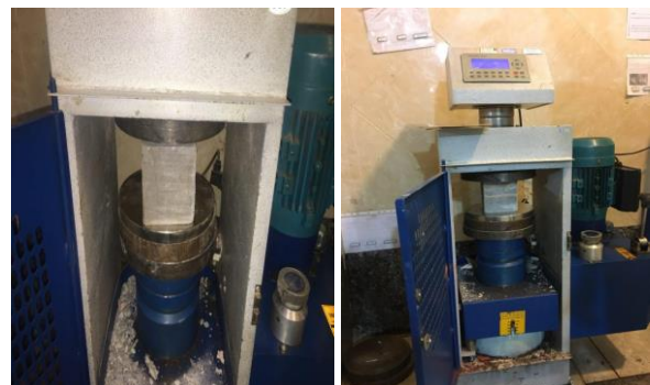
Fig. 3. Compressive strength test on RPC samples
