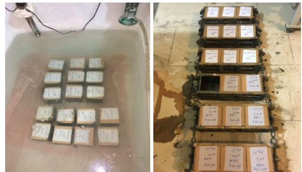
Fig. 2. (a) Prepared RPC samples, (with) wet curing in a saturated basin
