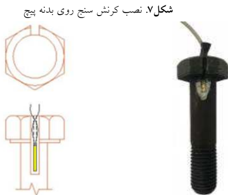
Fig. 7. Installation of strain gauges on bolt shanks
