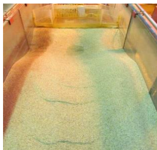
Fig. 3 Downstream view of scouring
