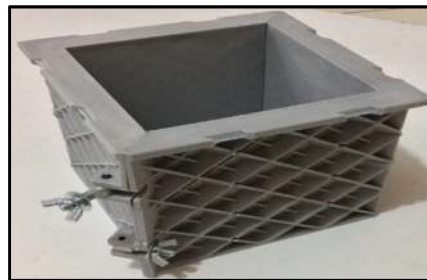
Fig. 3. The used template in making the product to check the sealing rate
