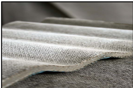
Fig. 1. Scheme of concrete canvas structure
