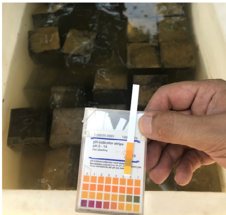
Fig. 3. Samples placed in magnesium sulfate solution
