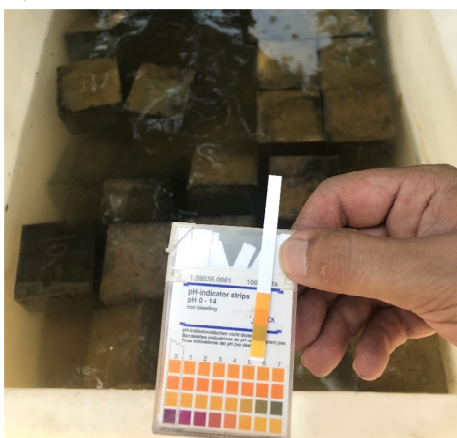
Fig. 3. Samples placed in magnesium sulfate solution
