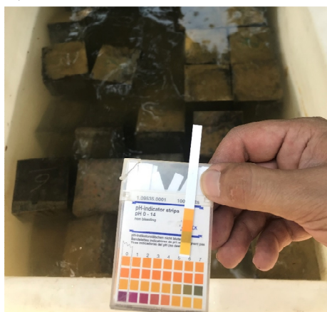
Fig. 3. Samples placed in magnesium sulfate solution
