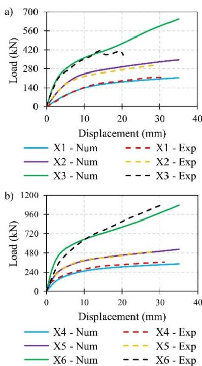
Fig. 5. Comparison numerical and experimental load-displacement curves.
