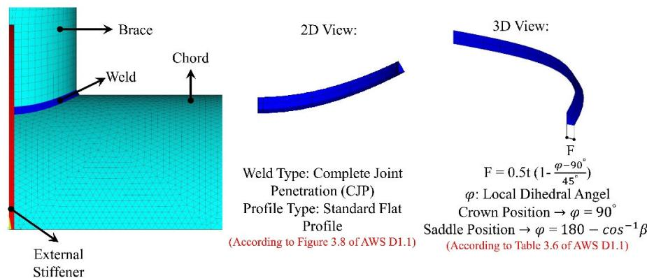
Fig. 2. Details of the modeled weld.
