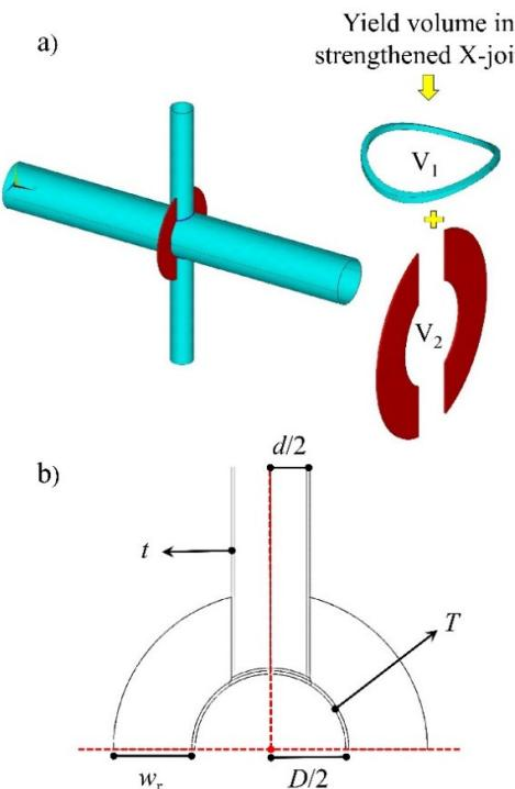
**Fig. 13.** a) Yield volume in stiffened and un stiffened joints, b) Calculation scheme to derive the relationship between the ratio of the ultimate strength of the stiffened joint to the ultimate strength of the corresponding unstiffened joint.
