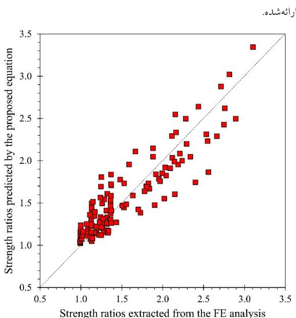
**Fig. 14.** Comparison of the strength ratios predicted by proposed equation with the strength ratios extracted from FE analysis.
