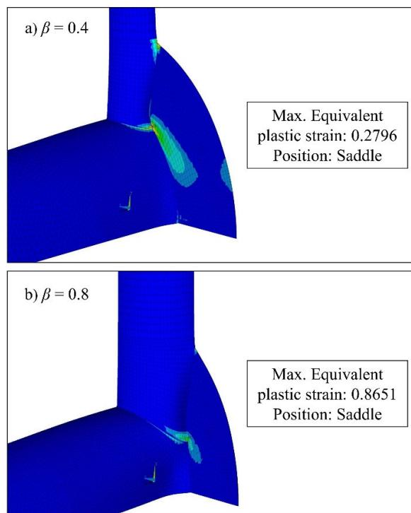
Fig. 8. The effect of the  $\beta$  on the equivalent plastic strain.
