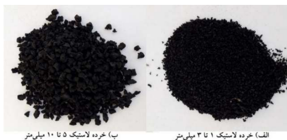
Fig. 1. Rubber crumbs used in concrete
