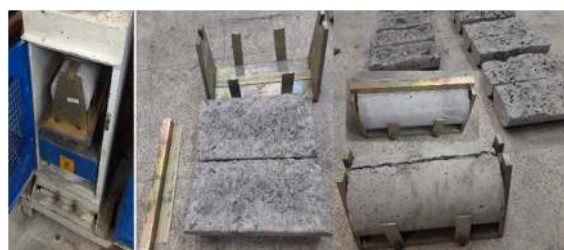
Fig. 7. Process and tools for tensile testing
