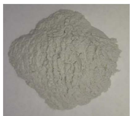
Fig. 3. Glass powder used to replace cement
