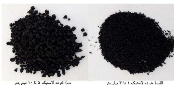
Fig. 1. Rubber crumbs used in concrete
