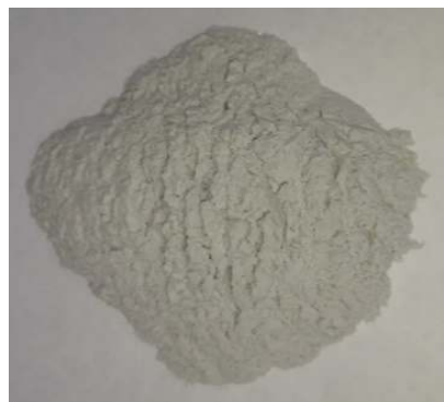
Fig. 3. Glass powder used to replace cement
