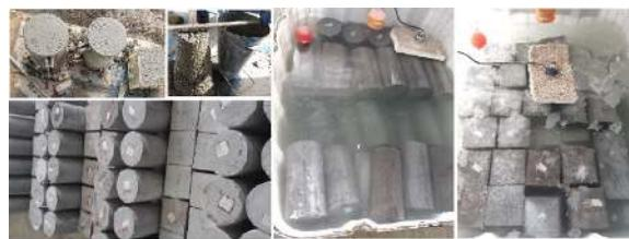
Fig. 4. Manufacturing, sampling, and curing processes of specimens
