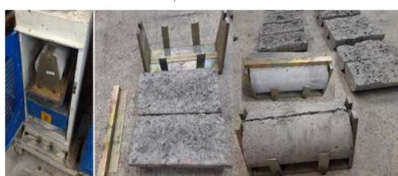
Fig. 7. Process and tools for tensile testing
