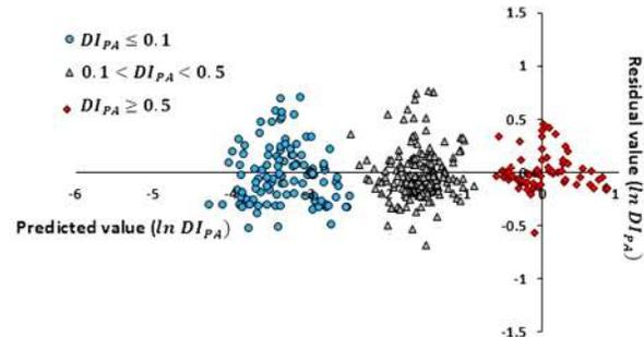
Fig. 6. Residual damage values (DI<sub>PA</sub>) against predicted damage values in TLM model and Intensity measure Sa(T<sub>1</sub>)
