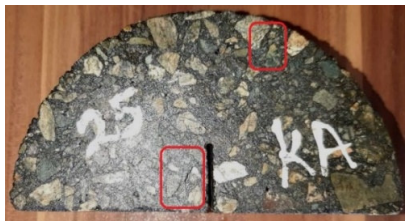
Fig. 7. Sample submerged in KAc
