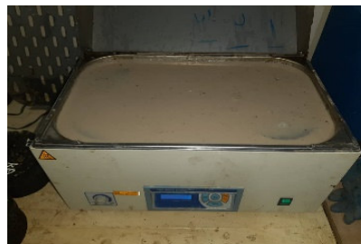
Fig. 2. Asphalt mixture conditioning in CMA
