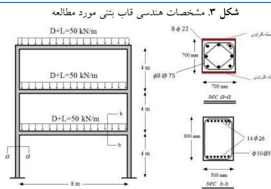
Fig. 3. Geometric properties of the reinforced concrete moment frame
