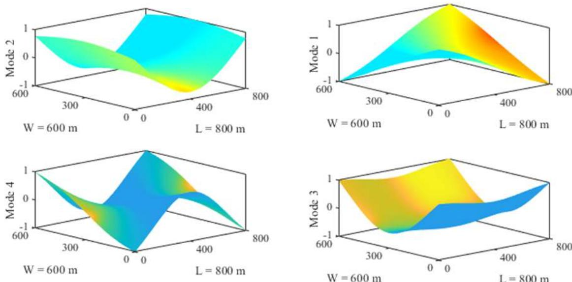
Fig. 2. Healthy mode shapes of the steel plate
