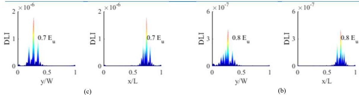
**Fig. 8.** 3<sup>rd</sup> mode DLI diagram of the D2 damage state with the damage severity (a) 10%, (b) 20% and (c) 30%
