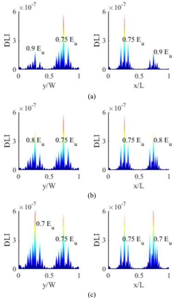
Fig. 10. 2<sup>nd</sup> mode DLI diagram of the D3 damage state with the damage severity (a) 10%, (b) 20% and (c) 30%
