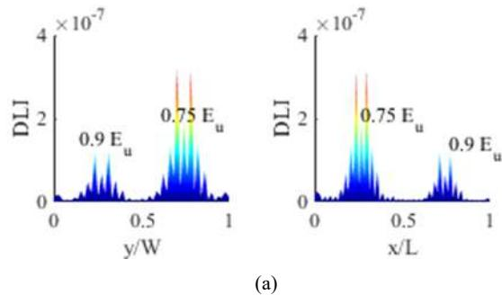
**Fig. 9.** 1<sup>st</sup> mode DLI diagram of the D3 damage state with the damage severity (a) 10%, (b) 20% and (c) 30%
