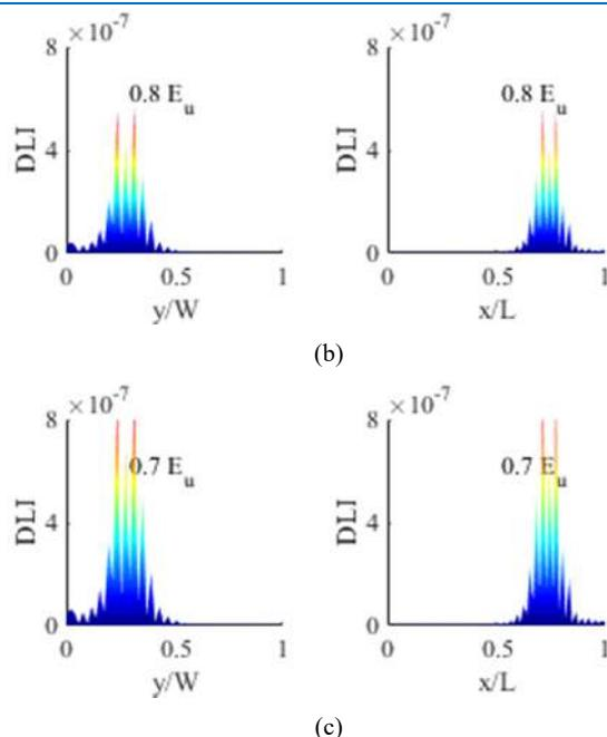
Fig. 12. 1<sup>st</sup> mode DLI diagram of the D2 damage state with the fixed support condisions and the damage severity (a) 10%, (b) 20% and (c) 30%
