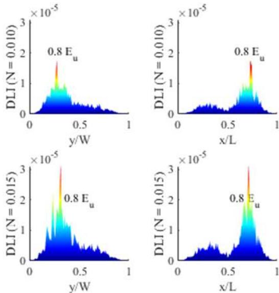
Fig. 13. 1<sup>st</sup> mode DLI diagram of the D2 damage state with the fixed support condisions and the effect of noise on mode shape signals
