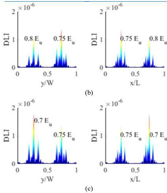
Fig. 11. 3<sup>rd</sup> mode DLI diagram of the D3 damage state with the damage severity (a) 10%, (b) 20% and (c) 30%
