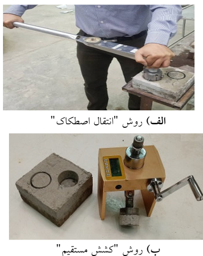
Fig. 4. Measurement of the shear and tensile bond strength between the mortar and concrete
