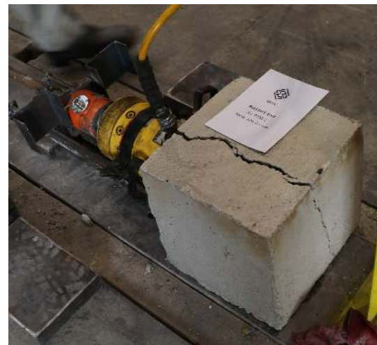
Fig. 9. Picture of split concrete (P25S-2) after test
