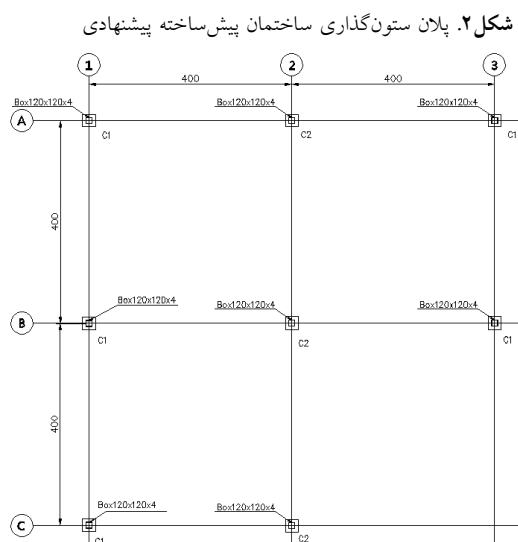
Fig. 2. Column plan of the proposed prefabricated building
