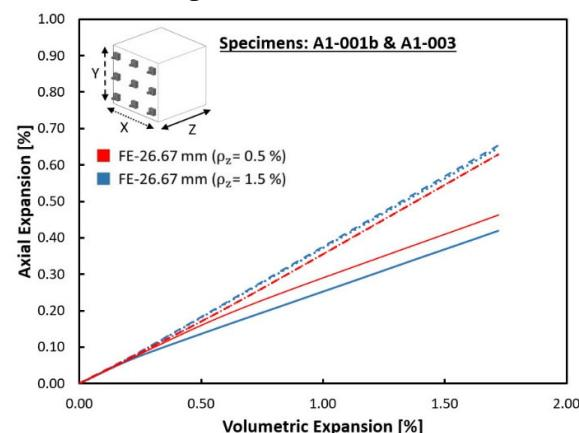
شکل ۱۲. Effect of reinforcement percentage on expansion distribution
