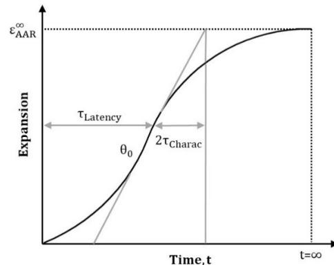
Fig 2. AAR-induced expansion based on Larive Model [32]
