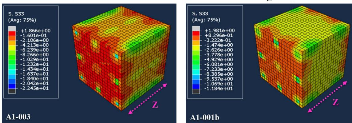
شکل ۱۳. Compressive stress level in concrete in the Z direction for Specimens A1-001b and A1-003 (in MPa)
