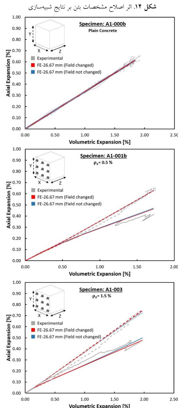
Fig. 14. Effect of modification of the concrete mechanical properties on expansion
