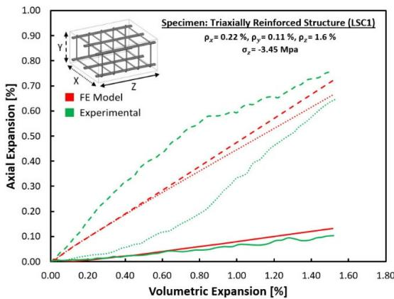
Fig. 20. Comparison of computed and measured results for the triaxially reinforced beam
