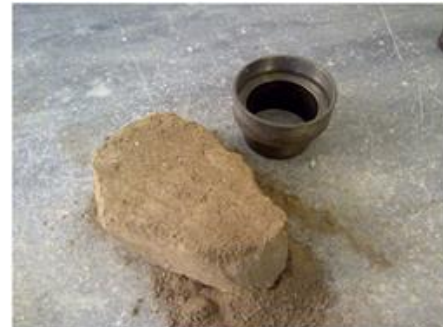
Fig. 5. Cut piece from obtained in-situ intact sample
