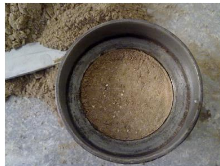
Fig. 6. Taking an intact sample with a sampler
