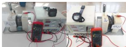
Fig 3. RCPT test according to ASTM C1202 standard
