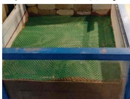
Fig 5. CE-121 geogrid used in tests
