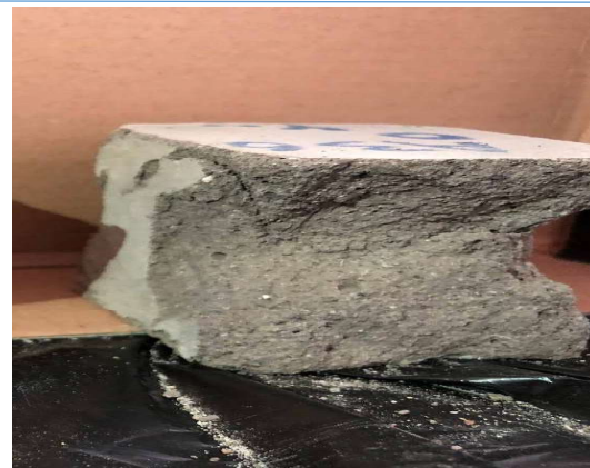
Fig. 10. The appearance of R2F12G0.5 design sample after 600 degree temperature
