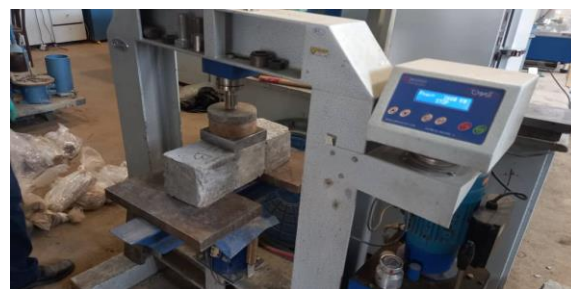
Fig. 4. Shear strength test
