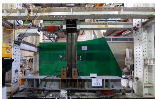
Fig. 8. Porposed self-centering connection test set up
