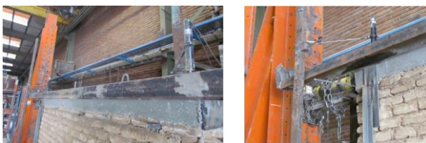
Fig. 10. Adopted instruments for measuring displacement
