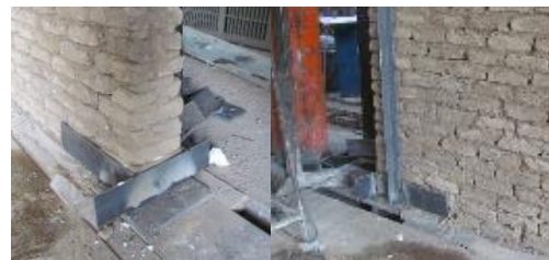
a) Controlling slip at heel and toe
