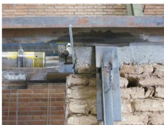
Fig. 13. Initiation of diagonal cracking
