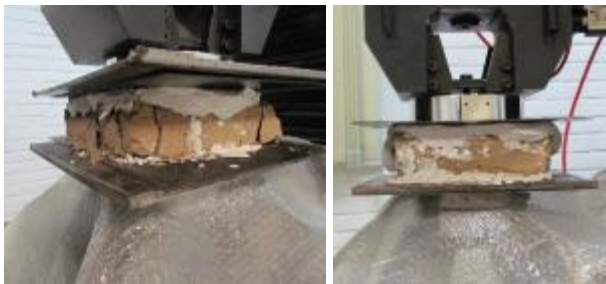
Fig. 5. Compressive strength test on adobe sample
