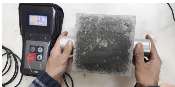
Fig. 9. Ultrasonic testing of the specimens
