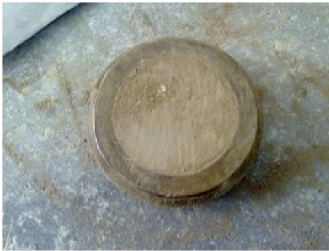
Fig 7. Transferring the intact specimen into the ring of the consolidation apparatus.
