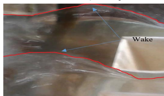
Fig. 4. Flow disturbance on the weir
