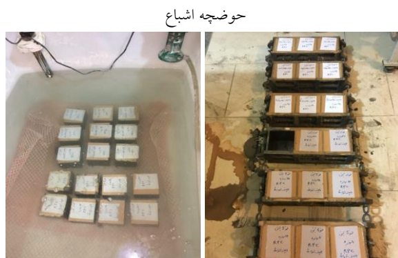
Fig. 2. (a) Prepared RPC samples, (with) wet curing in a saturated basin
