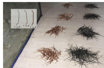
Fig. 1. Different types of steel fibers (groups 1, 2, and 3) with different specifications for making RPC samples
