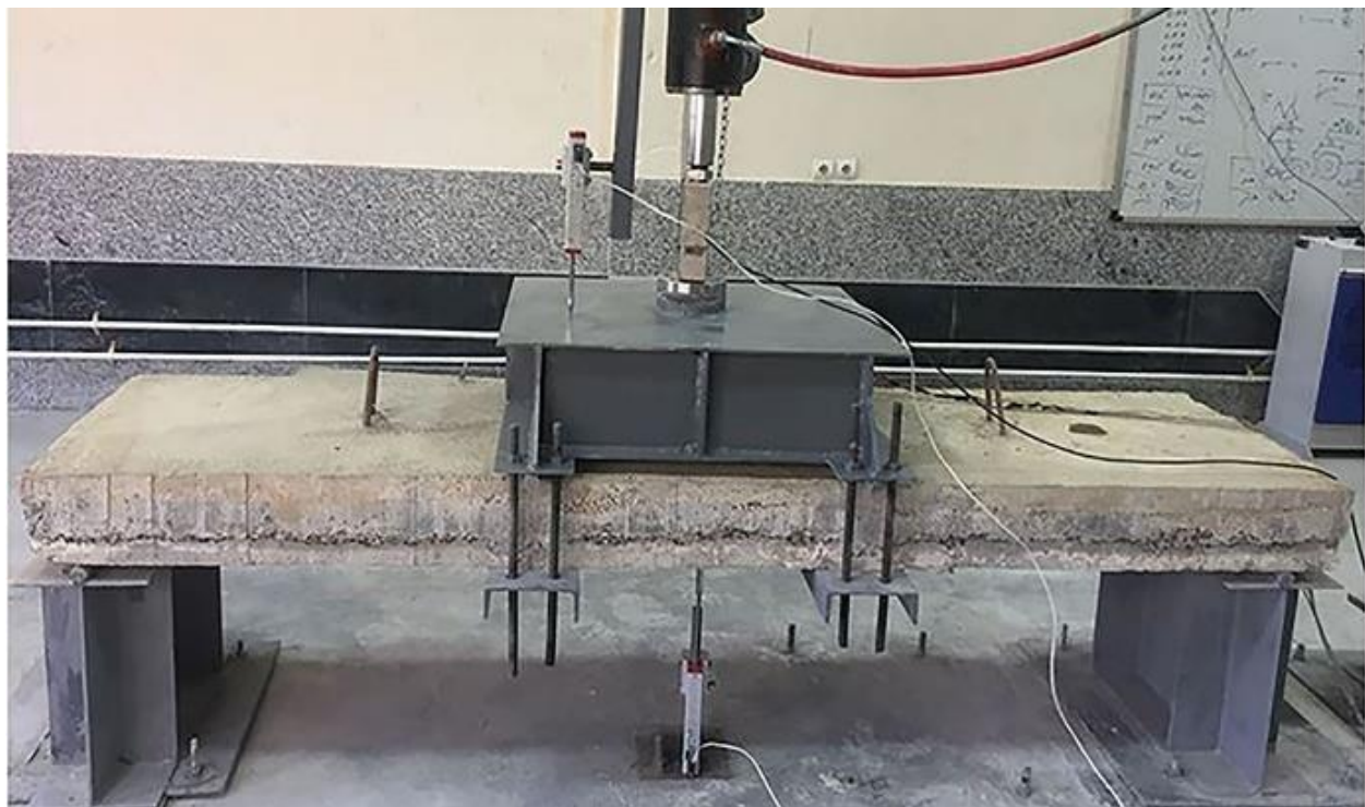
Fig. 5. Details of the flexural test setup of experimental specimens
