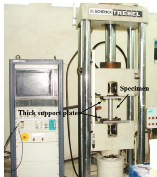
Fig. 2. Experimental setup for compressive test of the tubular column by Schenck machine.
