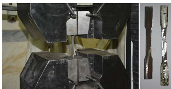
Fig. 4. Coupon specimen during the tensile test and after test completion
