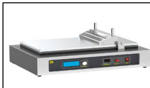
Fig. 2. Dr.Blade device for concrete canvas covering
