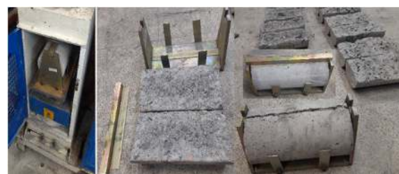
Fig. 7. Process and tools for tensile testing
