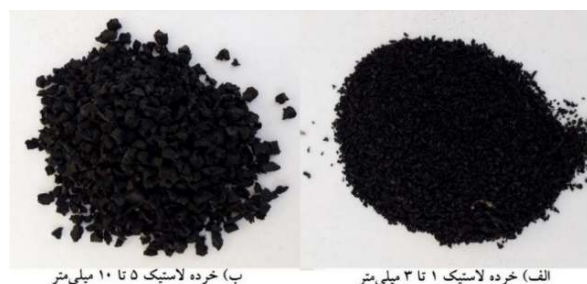
Fig. 1. Rubber crumbs used in concrete
